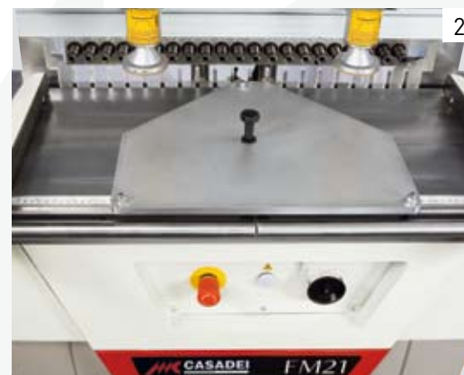
Photo 2: Fence for boring at 45°*
