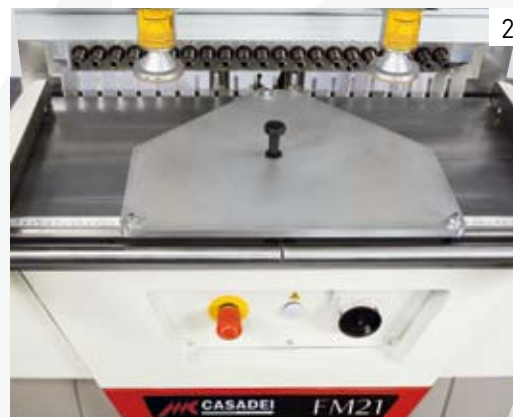
Photo 2: Fence for boring at 45°*
